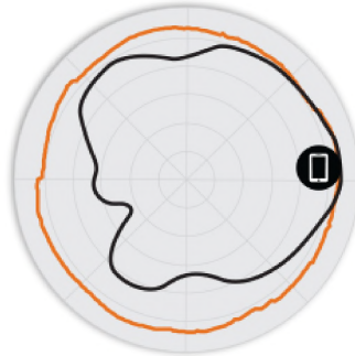
Figure 3. 5GHz Azimuth Antenna Patterns
